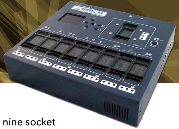
eMMC-F8 is a combination of programmer and duplicator, which is unique in the current market. It has nine socket sites; one is for programming the master IC and the other eight are for duplicating the slave ICs. The Master IC can be programmed with the files in the software (Dediware) while the slave IC can be duplicated with Master IC in stand-alone mode. With eMMC-F8, you will be able to program or duplicate on the same machine.
