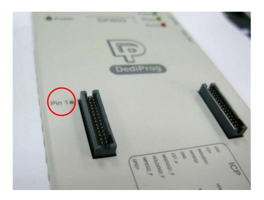
2. Ensure the triangle of socket to aim at the pin 1 position.
